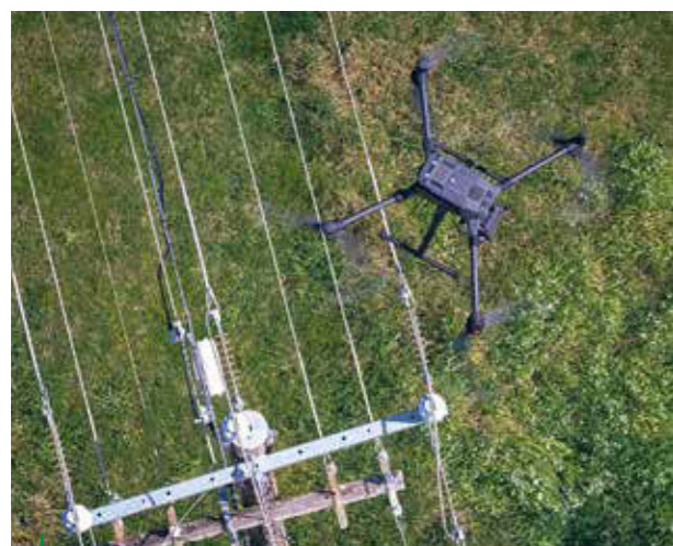
• Drones with powerful cameras and thermal imaging devices patrol powerlines across dense forest to keep network infrastructure safe from bush fire risk.
